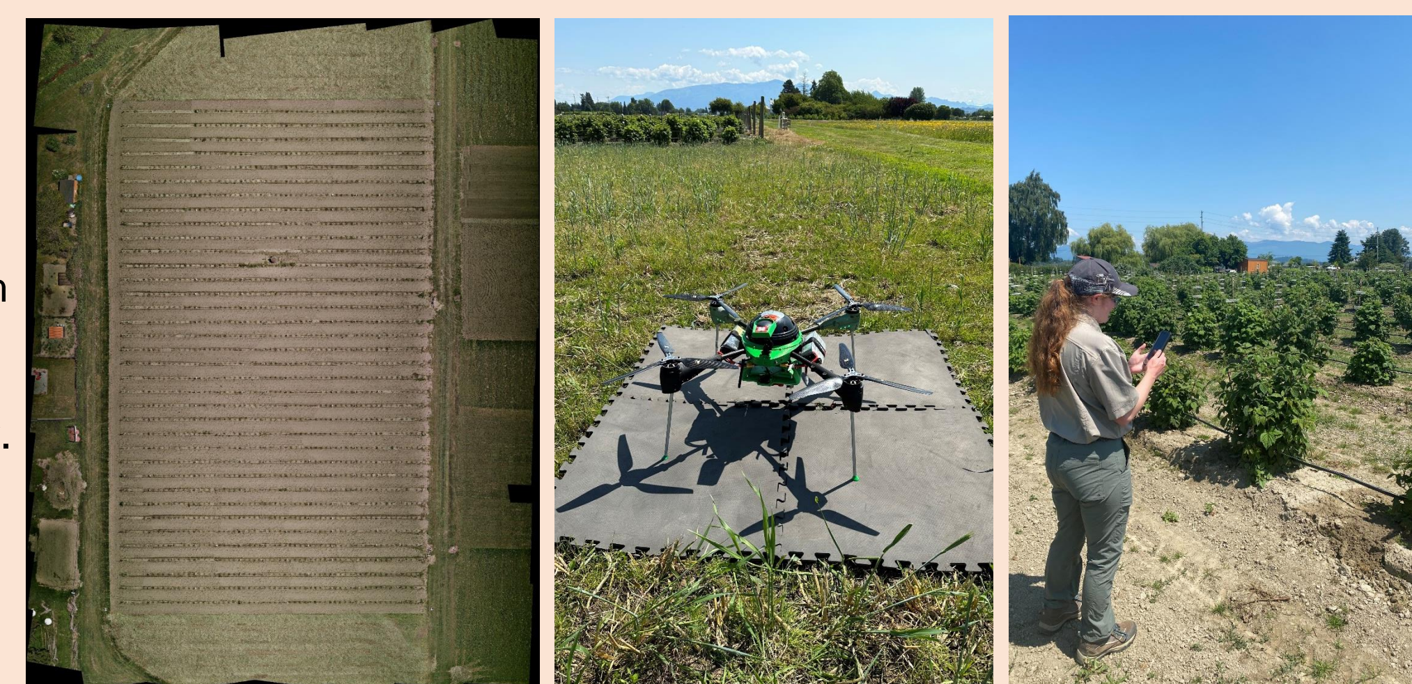
Figure 7 (right): Examples of ground-based and aerial imaging in action. A) Stitched red-green-blue aerial orthomosaic of field trial from May 5, 2023. Photo by Alexander Gregory. B) AgBOT mk 1 Quadcopter equipped with MicaSense RedEdge-MX multispectral sensor. Photo by Savannah Phipps. C) Savannah Phipps imaging in the AgerPoint Capture app with iPhone 14 Pro Max. Photo by Hannah Baker.
